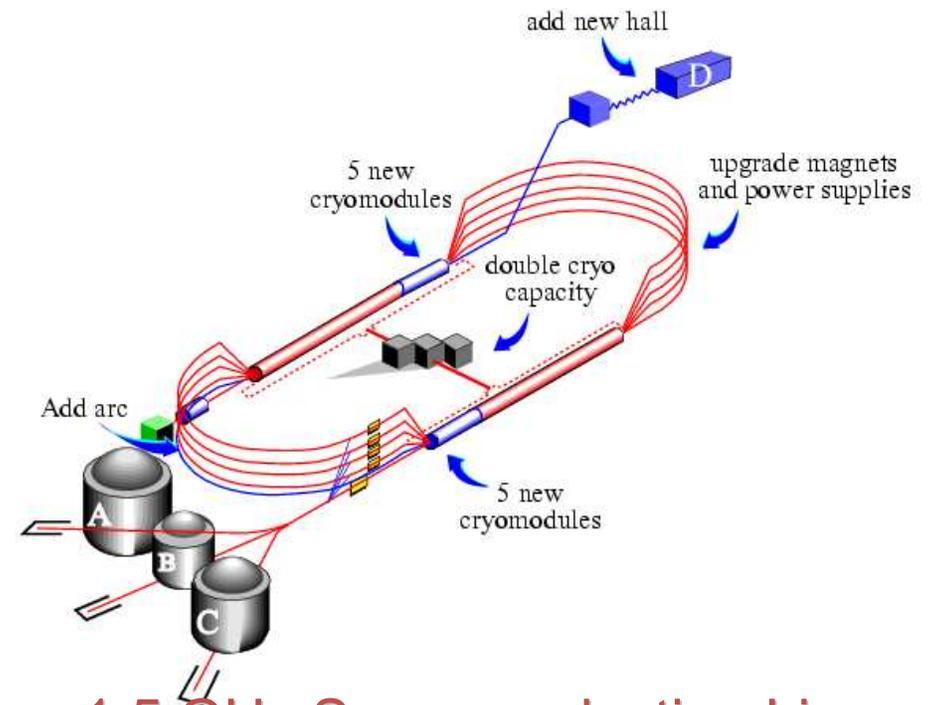
Two 1.5 GHz Superconducting Linear Accelerators provide electron beam for Nucleon & Nuclear structure studies.
