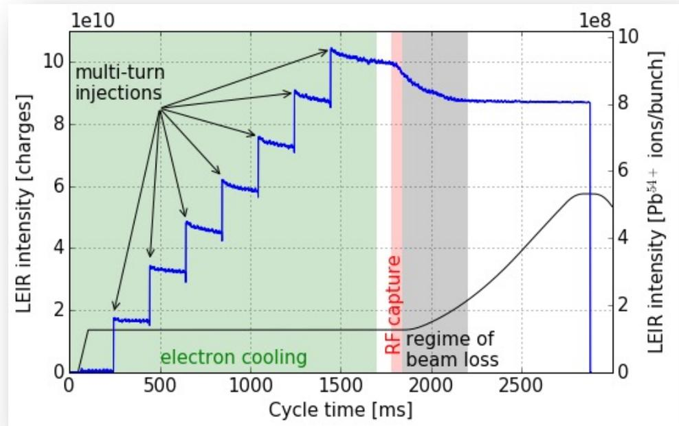
LEIR accumulates the 200  $\mu s$  pulses from Linac3; then it bunches the beam (1 or 2 or 3 bunches). Electron Cooling is used to achieve the required brightness. Acceleration to 72 MeV/nucleon (Pb) before transfer to the PS. LEIR Cycle is 2.4 s or 3.6 s.  $Pb^{54+}$  is fully stripped to  $Pb^{82+}$  in the transfer line from PS to SPS
