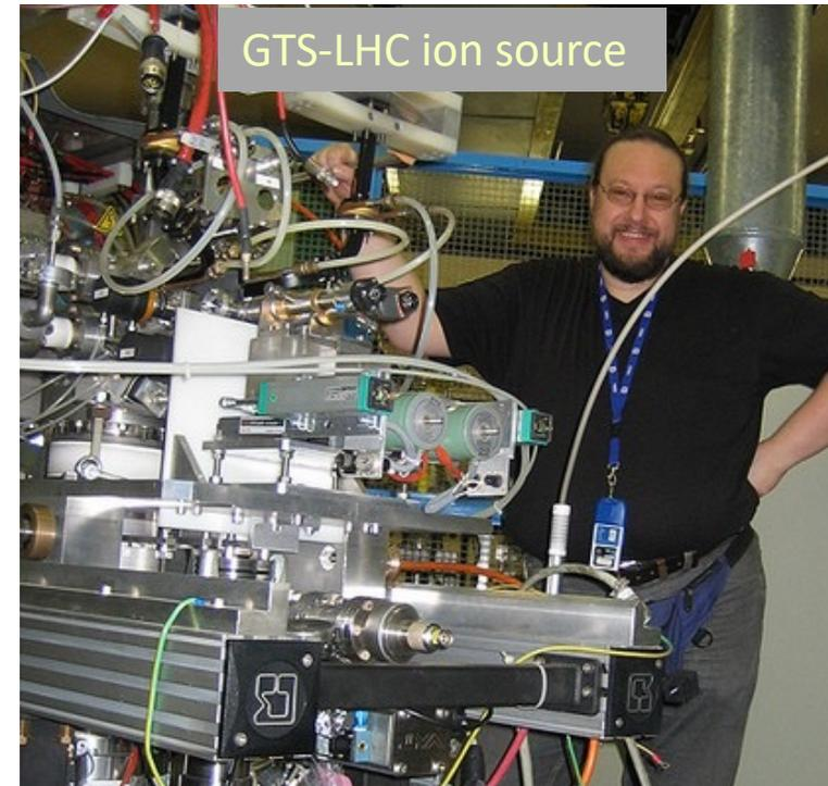
The metal is heated to around  $800^\circ\text{C}$  and ionized to become plasma. Ions are then extracted from the plasma and accelerated up to  $2.5\text{ keV/nucleon}$ .
