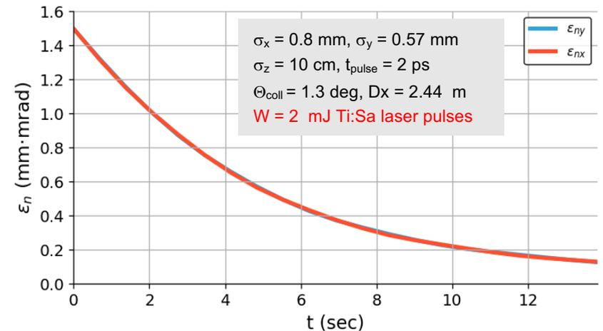
Simulation of laser cooling of the lithium-like Ca(+17) bunches in the SPS: **transverse emittance evolution.**
