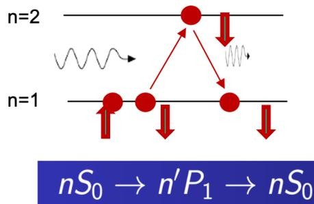
Closed transition in Helium-like atoms ( $n=1, n'=2$ ) preserve initial polarisation of the laser light
