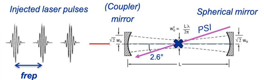
$$FSR = \frac{c}{L_{rt}} = f_{rep} = 40 \text{ MHz} \rightarrow L = 3.75 \text{ m}$$
