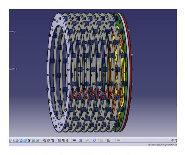
Fig. 26: CAD drawing of the TPC inner electrode structure.
