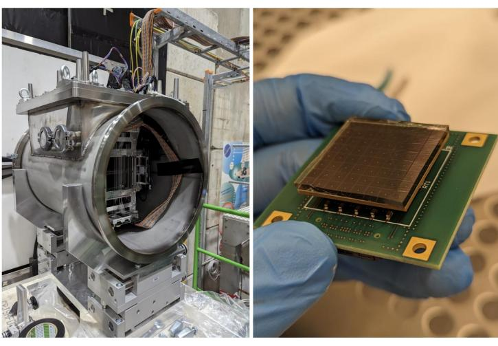
(a) UTS with SFH prototype in the target area. (b) Gel pad used to improve the SiPM-fiber coupling in the SFH prototype.
