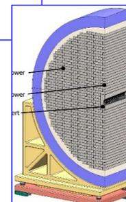
planar double amplification (GEM &  $\mu$ RWELL) modules & 2D-strip readout for the MPPGD outer trackers and disks
