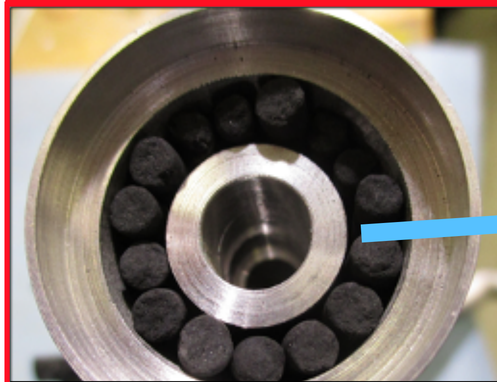
Cryo-vessel with charcoal.
