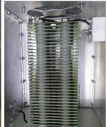
Air coil: 28.7 \mu H @ 871 kHz
