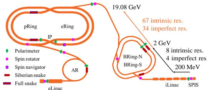
This constant-field snake has been simulation-verified and demonstrates **high hardware feasibility**, accommodating **rapid dipole ramping at 12 T/s** in the BRing-N.
