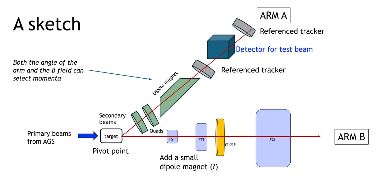
We can switch between A (test beam setup) or B (physics) or A+B (physics) on a movable platform
