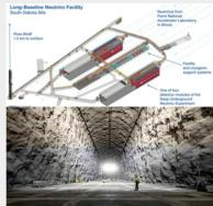
modules - tanks filled with liquid argon subjected to a uniform electric field.
