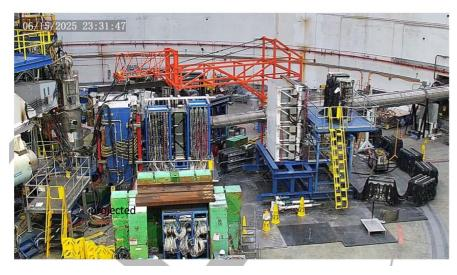
Recoil proton polarimeter
