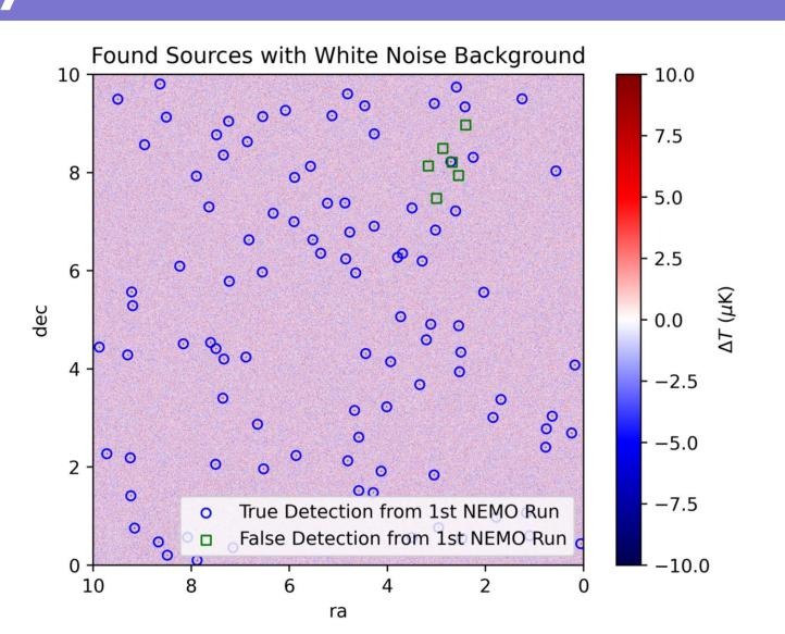
To characterize the effectiveness of source detection and subtraction, we use the output source catalog from Nemo to simulate a patch of sky and subtract that signal from the input patch. We then take the power spectrum of that source-subtracted map and take the ratio to the power spectrum of pure white noise (i.e. what would result from perfect subtraction).
