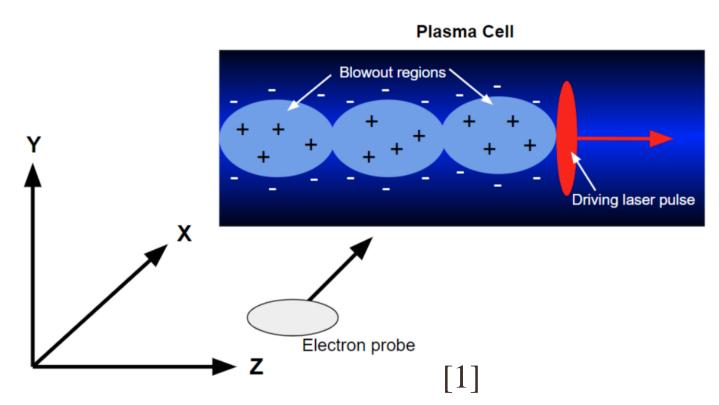
The plasma wakefield is modeled as a thin lens in the path of the probe electrons. This means that while passing through, the electrons will maintain their initial height and the forces acting on them will send them towards a focal point after they exit the
