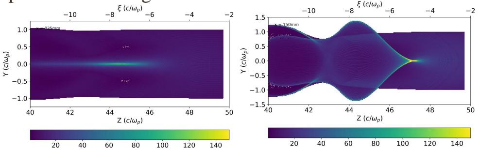
Simulation images of a full probe at distances x=25mm and 75mm behind the wakefield. The position with the highest density, later corresponding to the fastest expanding slice, is the position with the strongest focusing ( $\sim Z=44.5$ )
