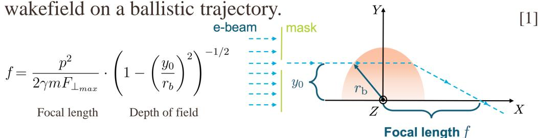
One issue with this is that electrons that enter the wakefield in different positions experience different focusing forces. Because electrons cross paths, it is useful to use masks to see where specific electrons go.
