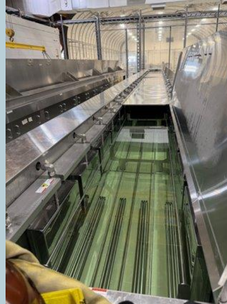
Ultrasonic Tank – Clean Room Assembly
