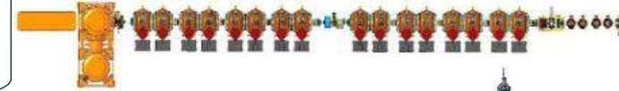
Low-Energy Cooler, IR02 - 16 197 QWR NCRF, 4 591 NCRF, 1 24 MHz NCRF, And 1 591 MHz Deflecting Cavity
