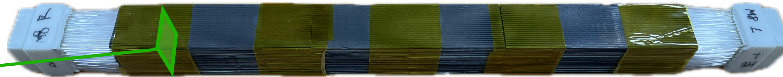
Pb/Sci module (30 mm x 30 mm x 320 mm, 4x8 units)
